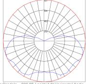
Maximum Candela = 926.88 Located At Horizontal Angle = 0, Vertical Angle = 65 #1 - Vertical Plane Through Horizontal Angles (0-180) (Through Max. Cd.) #2 - Horizontal Cone Through Verticle Angles (65) (Through Max. Cd.)
