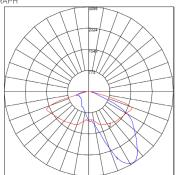
Maximum Candela = 3098.323 Located At Horizontal Angle = 60, Vertical Angle = 67.5 #1 - Vertical Plane Through Horizontal Angles (0-180)
