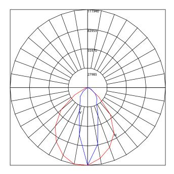
Maximum Candela = 111939.5 Located At Horizontal Angle =-10, Vertical Angle = 0 H - Horizontal Axial Candela V - Vertical Axial Candela
