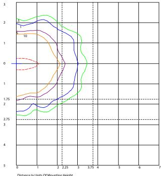
Distance In Units Of Mounting Height Values Based On 10 Meter Mounting Height 1/2 Maximum Candela Trace Shown As Dashed Curve (+) = Maximum Candela Point
